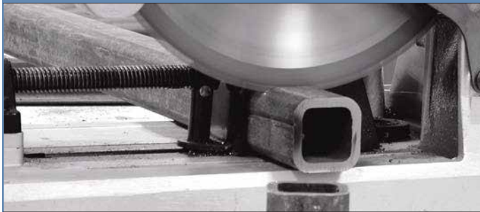
Carbide-Tipped Blades make Virtually Spark-Free Cuts
