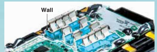
Terminal short-circuit prevention structure
